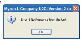
If there is a problem and the download process cannot be started within the instrument's automatic timeout period, the U2CI will display a message indicating there is no response from the instrument. In this case, put your instrument back into "PC On" mode and try again.
