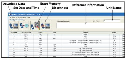
**UMII Commands:** You may use the icon buttons (shown above) or the UMII Commands drop down menu to send commands to the instrument.
