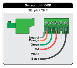
**NOTE:** It is suggested that the user mount watertight restraint fixtures and at least one service loop on all cabling. All cabling should be routed using best practices to protect from damage and/or electromagnetic interference (EMI). Consider grounded steel conduit for maximum protection. Signal cables should be routed separate from line power cables or any other source of interference.
