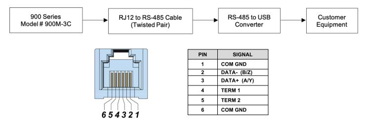
To enable cable line termination on the last unit, short TERM 1 to TERM 2. NOTE: If you use terminations, they must be applied to both ends of the cable.
